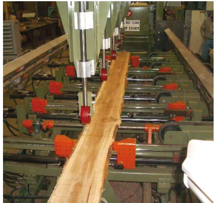
Infeed of the Crosby edger showing the holddown rolls, the dogs and the infrared profilers
